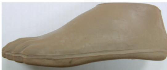
Figure 5. The modified natural rubber CR SACH foot.
