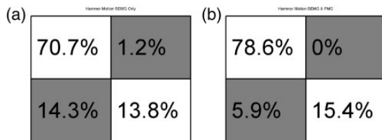
Figure 8. Confusion Matrix reporting classification results for radial and ulnar deviation of the hand: (a) 4 SEMG inputs; (b) SEMG and FMG inputs.
