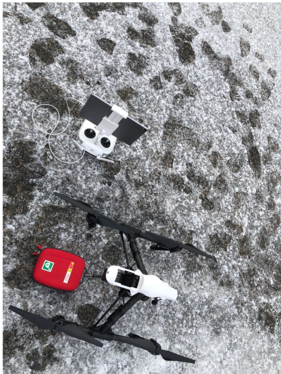
Fig. 5 Photo of iPad (that provided live video streaming), drone and AED. Photo of iPad (version 3) that provided live video streaming, drone (a modified DJI Inspire 1) and AED (Schiller FRED easyport™) that were used during simulations
