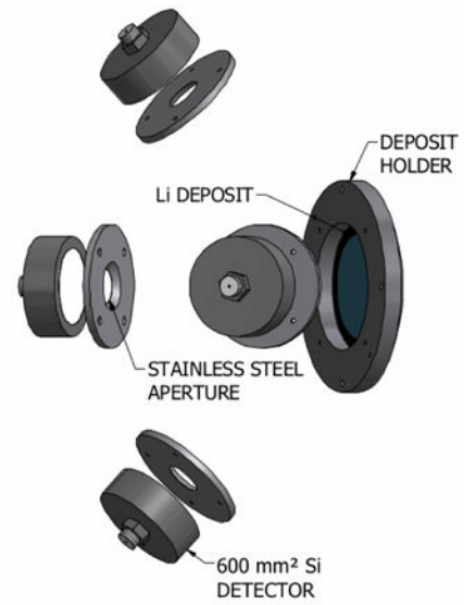
Figure 3. Illustrations of (a) a section view of the neutron monitor vacuum chamber and (b) a representation of the detection geometry.
