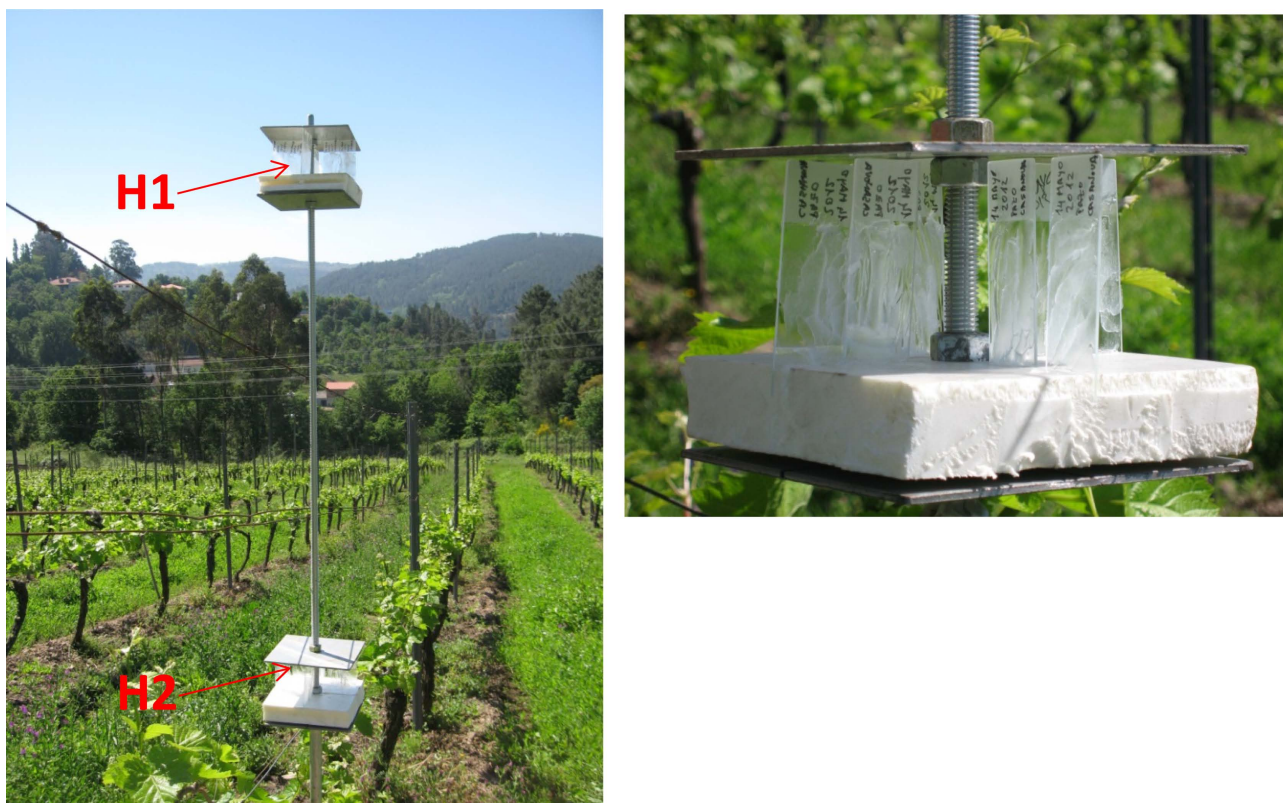
Fig. 2. Airborne sporangia capture using sticky glass traps facing N, S, E and W. Two supports (A and B) were placed in each plot (at different altitudes if possible), and the traps they carried at two heights (H1 and H2 m) above the soil.
