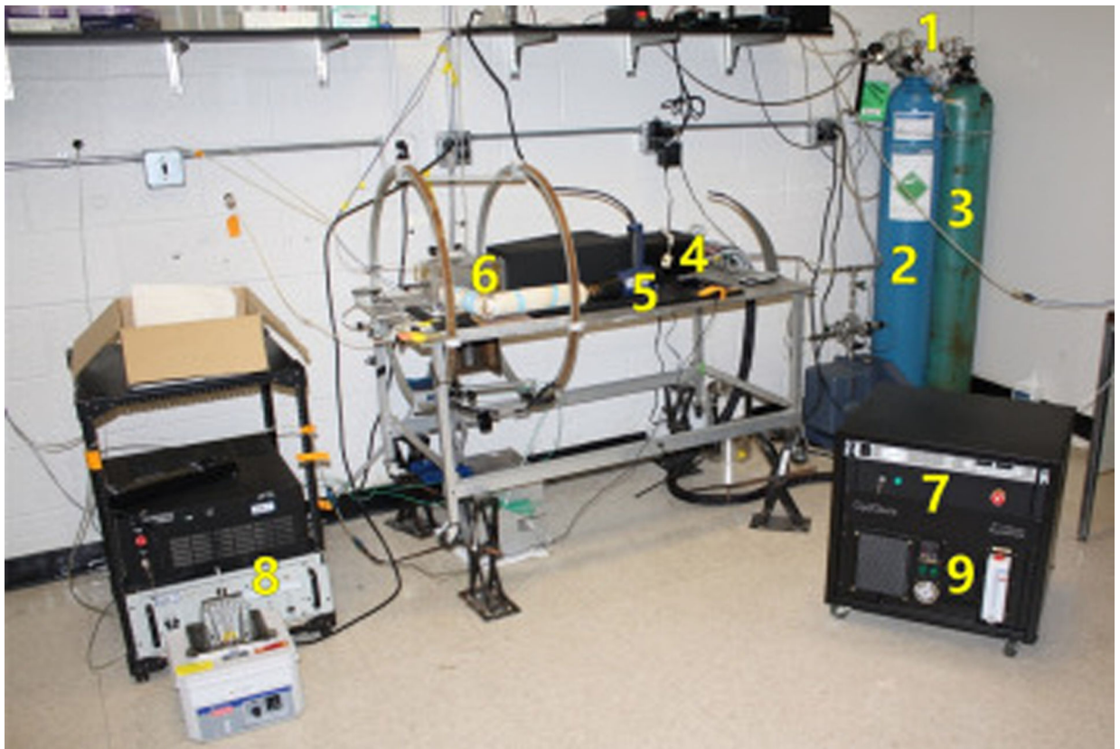
Fig. 6. Overview of a home-built ^{129}\text{Xe} hyperpolarizer. (1) Pressure gauge A; (2) Xe gas mixture tank; (3) N 2 tank; (4) laser; (5) heat gun; (6) Rb cell; (7) laser control panel; (8) magnet (Helmholtz coil power supply); (9) chiller.
