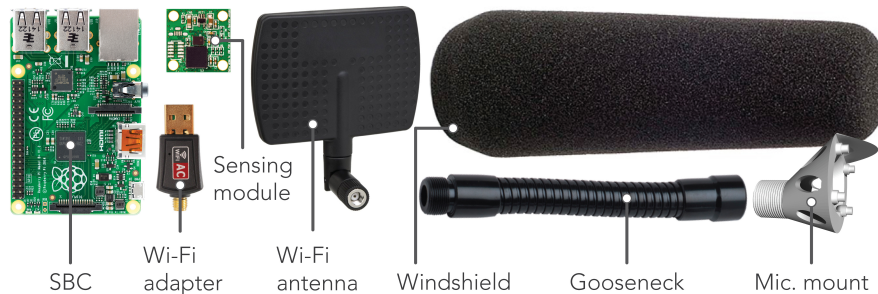
Figure 4. Main part list for complete node at relative scale (excluding housing).
