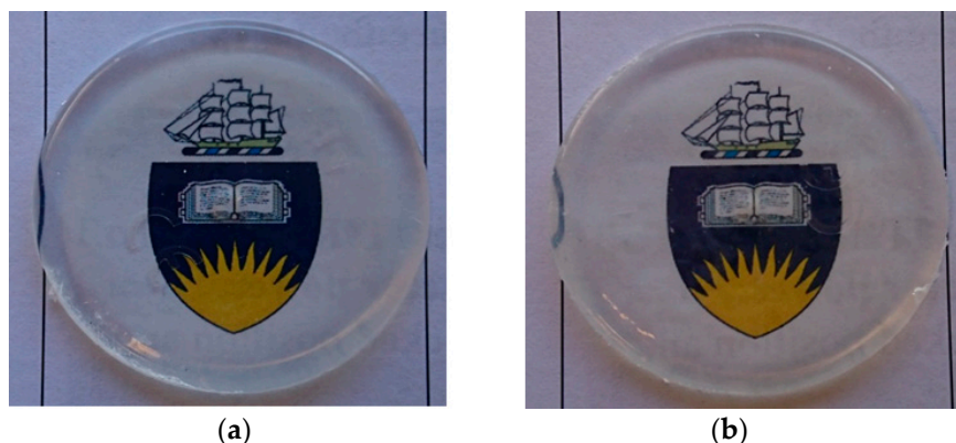
Figure 8. 50/50 + 5 wt % glycidyl methacrylate (GMA) composition after two-step polymerisation: (a) 1 layer and (b) 3 layers.
