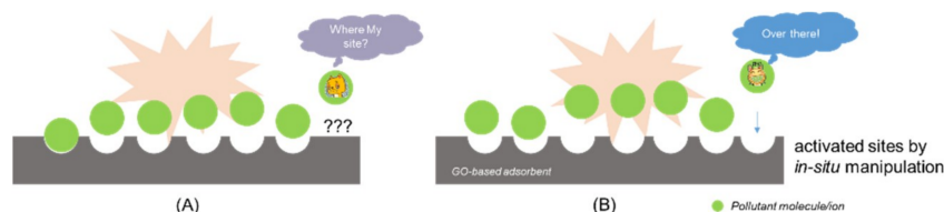
Figure 8. (A) The schematic diagram of conventional one-step adsorption; (B) Enhanced two-step adsorption: simultaneously generate new sites from inactive structures for enhanced capacity.
