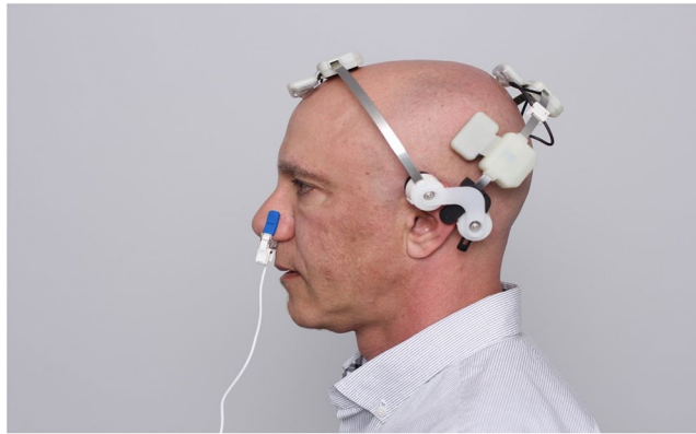
Figure 2. The Vielight Neuro Gamma in use. The stimulation modules consist of a Nasal Applicator, and a Head Set with four light emitting diode (LED) modules intended to be positioned over the hubs of the default mode network (DMN).
