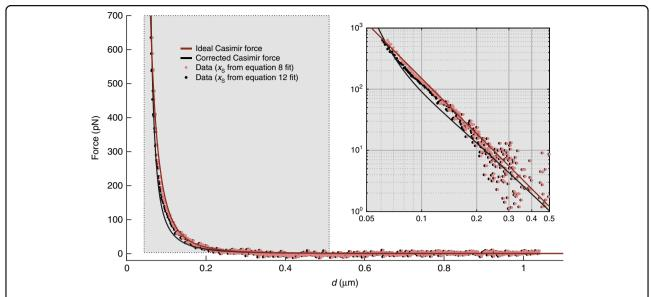
Fig. 3 Casimir force measurements compared with ideal theory (Eq. 8) (red) and theory for real metals (Eq. 12) (black). Inset shows the highlighted section of the data in log-log scale for better comparison between data and theory at small separations. The two sets of data are identical but shifted by 2 nm along the abscissa because of the different values of  $x_s$  returned from the fits to Eqs. 8 and 12
