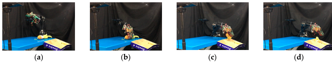
Figure 51. A procedure of grasping the fifth object: (a) The target object (low stiffness category); (b) Collision-free paths for grasping; (c) RRT-Connect algorithm; (d) Successfully separated and placed in different boxes.
