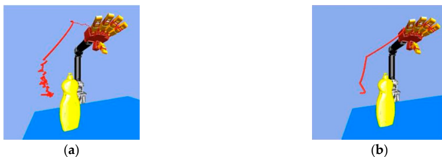
Figure 17. Path pruning algorithm: (a) Original path; (b) The path through path pruning algorithm.
