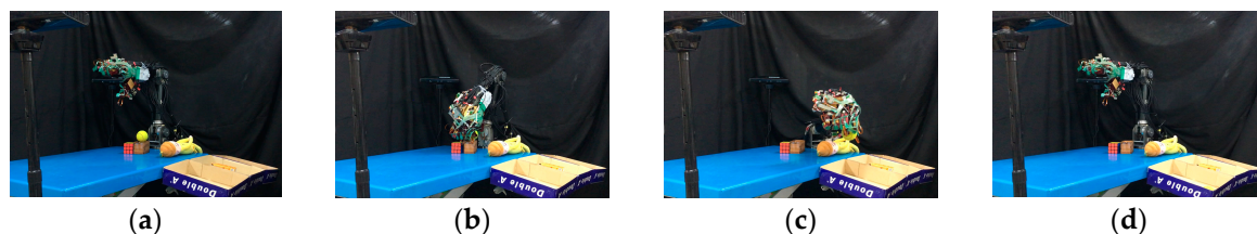
Figure 42. A procedure of grasping second object: (a) The target object (top box); (b) Collision-free paths for grasping; (c) RRT-Connect algorithm; (d) Successfully separated and placed in different boxes.
