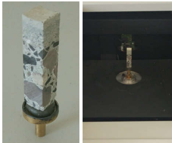
Figure 27. Sample mounted on base and placed in microtomograph chamber.
