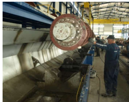
Figure 2. Steel mould with attached little mould is being placed in centrifuge.
