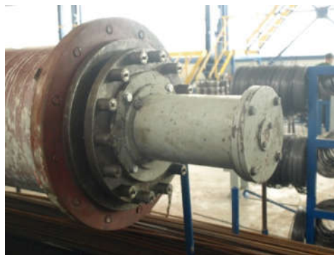
Figure 1. Little mould attached to steel mould used for manufacturing spun concrete power poles.
