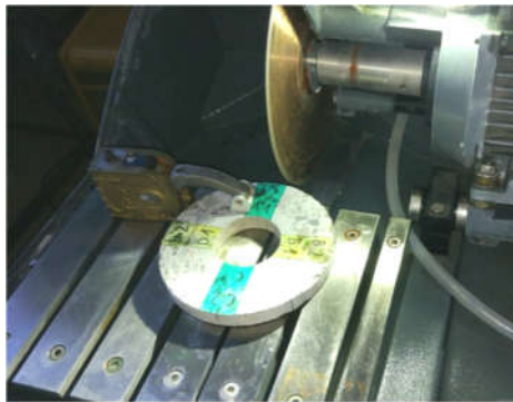
Figure 4. The slice mounted in the chamber of precision saw.
