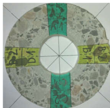
Figure 3. About 10 mm slice cut out of principal sample. Division of slice into smaller samples for tests proper is shown.
