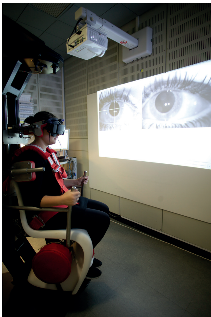
Figure 1. The TRV chair setup. The patient is fixed in the chair and fitted with videonystagmography goggles. Eye movements are presented on the wall monitor.
