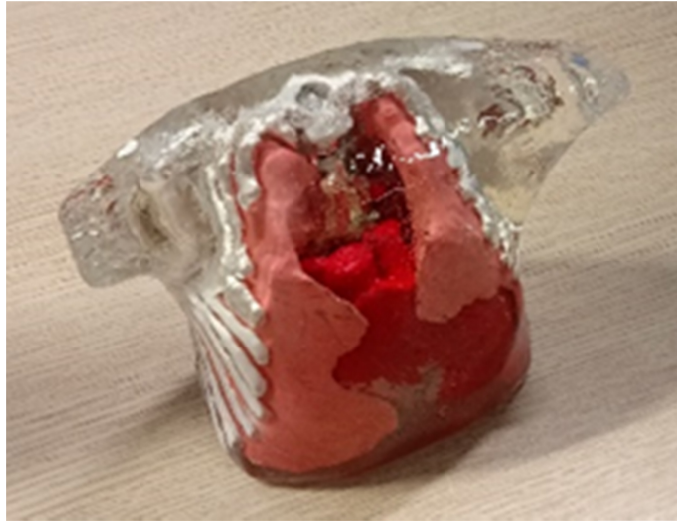
Fig. 5. Non-scattering anatomically correct 3D mock-up SiliGlass phantom made using CT scans of a newborn infant.
