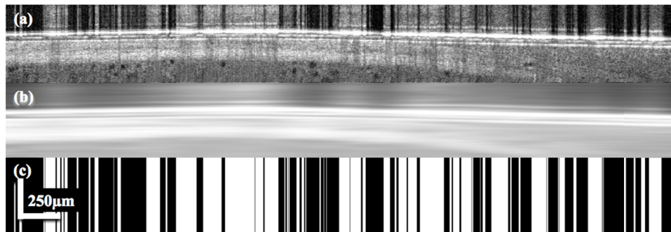
Fig. 6. (a) Original section of B-scan with high reflection. (b) Section of the same high reflection B-scan following application of a horizontal blurring filter. (c) Binary mask with all white portions representing all A-scans in 6a whose mean intensity value exceeded 15 above the mean intensity value of the corresponding A-scan in 6b. (49% of A-scans in this example qualify as reflection stripes)
