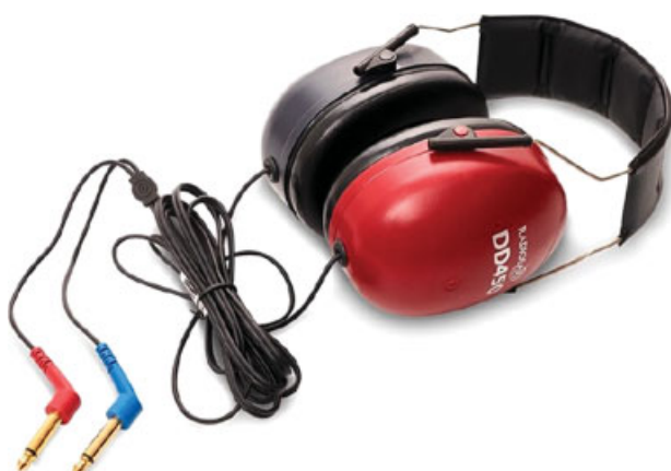
Figure 2 Circumaural headphones can be used for standard and extended high frequency air conduction audiometric testing.
