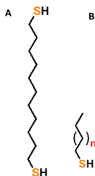
Figure 4. Panel (A) is the linker (SHC 11 SH) and (B) represents the diluent molecules ( n = 1, 3, 5, 7 respectively for C 4 SH, C 6 SH, C 8 SH, and C 10 SH).
