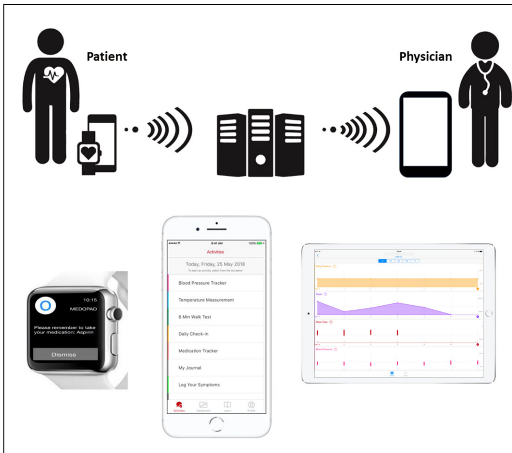
Figure 1 Cardio patient monitoring platform. Self-measured physiological data and further patient-reported outcome parameters are entered daily by the patient. Together with activity data from the Apple HealthKit, the information is transmitted via a secure immediate worldwide Internet-based transfer to the treating physician.
