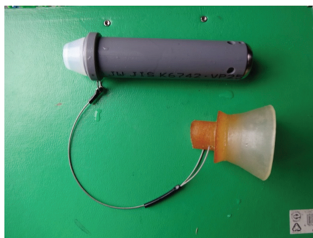
Figure 1. Photograph of the indwelling ruminal pH sensor (160 mm in length and 32 mm in diameter) connected to the cover of the rumen cannula by a cord. The sensor was specifically developed for calf research based on a radio transmission pH measurement system in adults (Sato et al., 2012).
