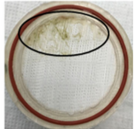
Figure 2: Photographs of a typical bundle inlet and outlet (top row) and that of Trial 4 (bottom row) at explant. Circle indicates area of clot formation
