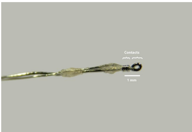
FIGURE 1 Bipolar electrode for dorsal root ganglion stimulation. Bipolar DRGS electrode. The insulation from the terminal portion of the larger wire was removed, and the terminal portion of the wire was folded back upon itself to produce an atraumatic tip. The insulation was similarly removed from the end of the smaller gauge wire, which was then wrapped helically around the insulated portion of the central wire (see reference [18]). Both the anode and the cathode were implanted at the L5 DRG [Colour figure can be viewed at wileyonlinelibrary.com ]
