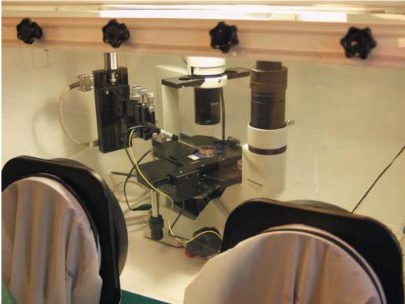
Figure 1. The set-up for measuring oxygen tension is shown in place inside the incubator. The oxygen microsensor is held by a motorized micromanipulator mounted on a metal frame on the inverted Olympus CK41 microscope.
