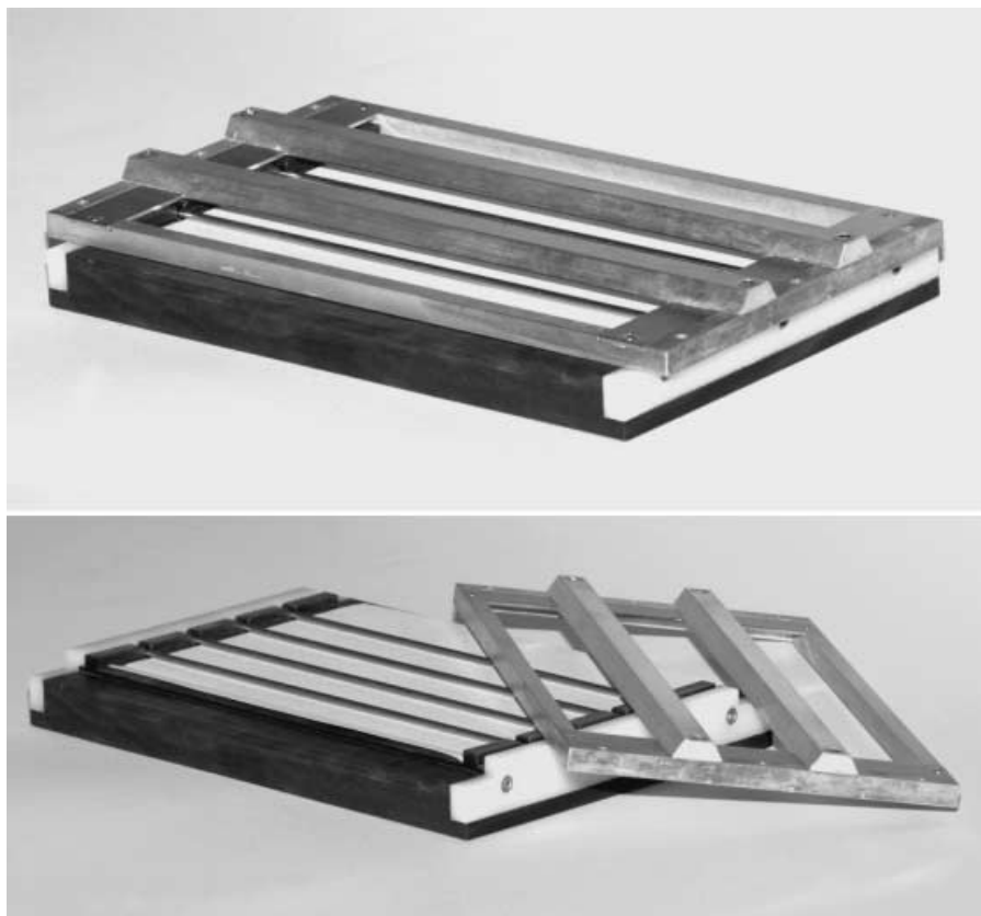
Figure 2. The gut-cutting device. Shown with the lid on or off. Note the rods placed in their grooves.
