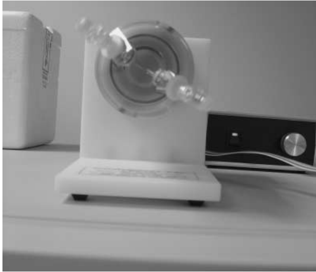
Figure 5. Synthecon microbioreactor for sustained three-dimensional generation of tissues, such as hepatic tissue illustrated in Fig. 1.
