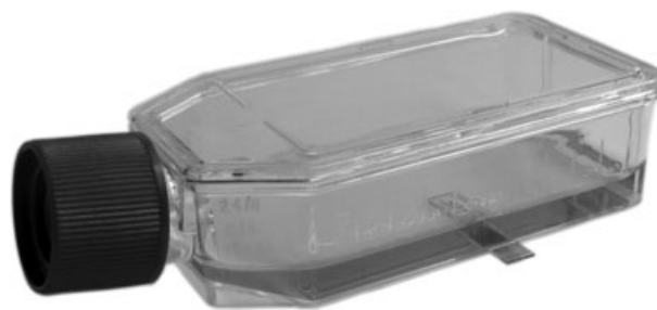
Figure 1. Sensing Cell Culture Flask: the transparent sensor chip is embedded in a conventional tissue culture flask.
