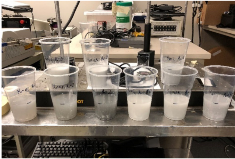
Figure 1. 9 solid phantoms with different optical properties inside the curing molds.
