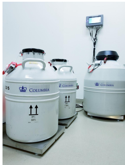
Fig. 1 Experimental set-up. LN 2 dewars equipped with temperature probes were placed on scales. Weights were recorded continuously in real-time via relay to an Ethernet-connected monitoring unit
