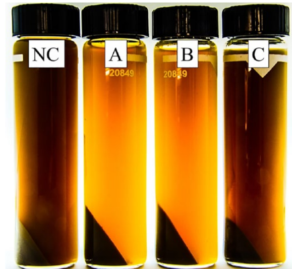
Figure 2. Oral fluid specimens following treatment. NC = negative control; A = formula A (chitosan 100 ppm, Tween 20 0.1%, BSA 0.5%, xylene cyanol 1 ppm); B = formula B (chitosan 100 ppm, BSA 0.5%, xylene cyanol 1 ppm); C = formula C (Tween 20 0.1%, BSA 0.5%, xylene cyanol 1 ppm).
