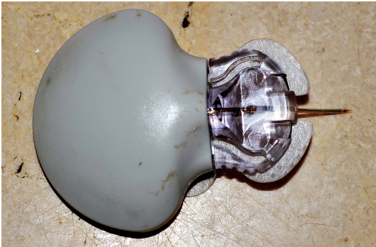
Image 4: Continuous blood glucose monitor sensor and transmitter. This is a representative continuous blood glucose monitor, composed of two parts: a transmitter (left side opaque portion of device) and a sensor (clear plastic with subcutaneous catheter). The sensor catheter is inserted in the subcutaneous tissue and secured with an adhesive strip. This particular device transmits blood glucose readings directly to an insulin pump.
