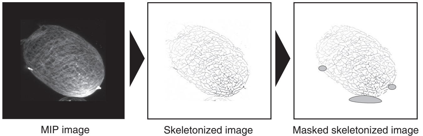
FIGURE 2 Workflow of image processing steps for obtaining the images used to derive the metrics to quantitatively evaluate cellulose network configuration
