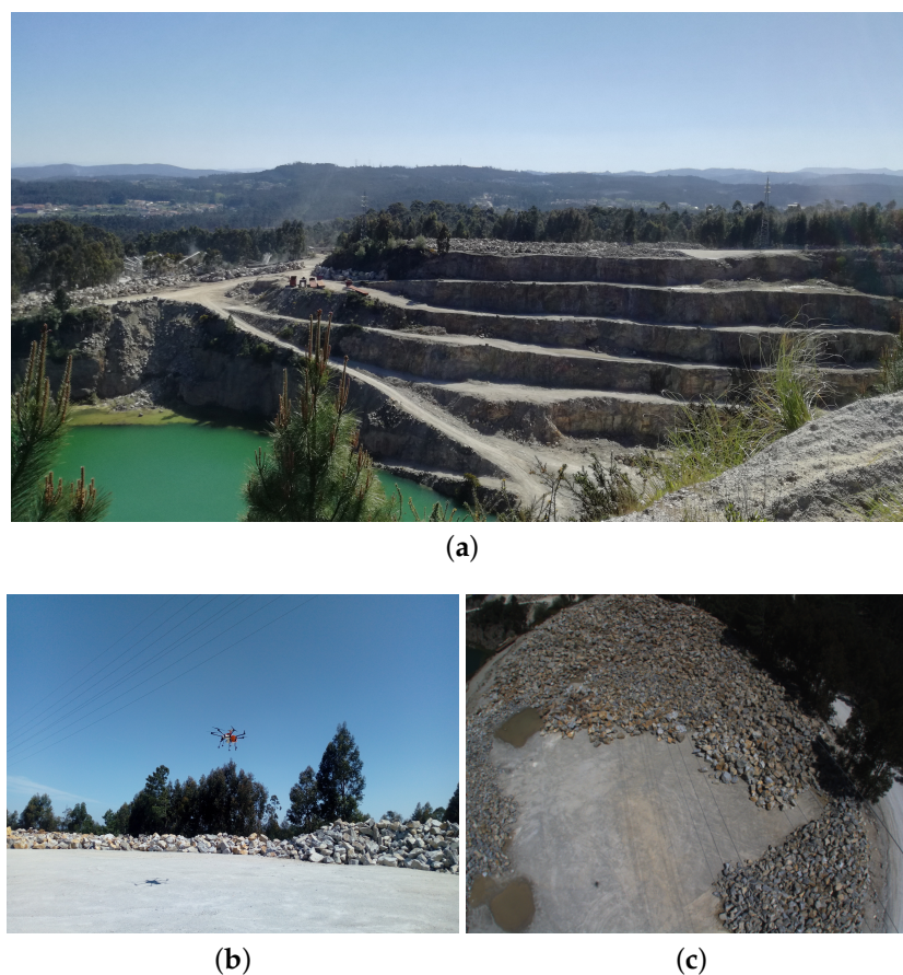
Figure 10. (a) Malaposta quarry overview; (b) STORK UAV mapping the stockpile; and (c) STORK UAV onboard images.
