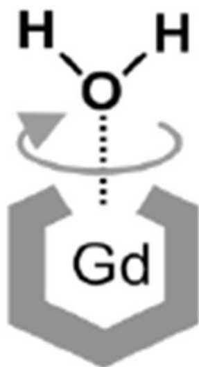
Figure 31: Restricting the water ligand mobility (specifically rotation about the Gd-O bond), in Gd(III) complexes through interaction with an intramolecular H-bond acceptor. Reproduced with permission from Ref. 123 ( URL: http://dx.doi.org/10.1002/anie.201702274 ). Copyright 2017 John Wiley and Sons.
