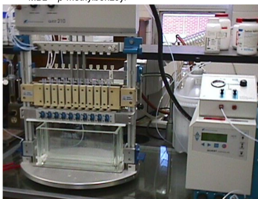
Scheme 24. Solution Phase Automation of the Oligosaccharide Synthesis in One Pot Using Parallel Synthesizer Quest 210 a
