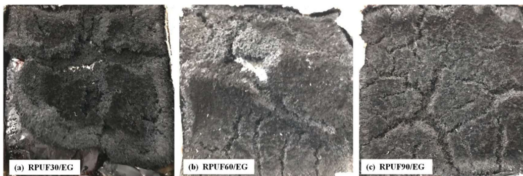
Figure 10. Digital images of RPUF/EG after cone test: (a) 30 kg/m 3 , (b) 60 kg/m 3 , (c) 90 kg/m 3 .
