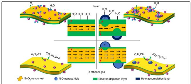
Fig. 5 Ethanol sensing mechanisms of pure and NiO-decorated SnO nanosheets. Schematic illustration of ethanol sensing mechanisms of pure (left) and NiO-decorated (right) SnO<sub>2</sub> nanosheets
