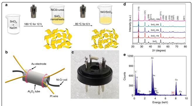
**Fig. 1 Synthesis of NiO-decorated SnO nanosheets. a** Schematic illustration of the synthesis route for NiO-decorated SnO<sub>2</sub> nanosheets; **b** Schematic diagram and **c** photograph of the as-fabricated sensor; **d** XRD patterns of the synthesized samples of pure SnO<sub>2</sub> and NiO-decorated SnO<sub>2</sub> nanosheets with NiO concentrations of 1, 3, 5, and 10 mol%; **e** EDX spectrum of SnO<sub>2</sub>-3Ni
