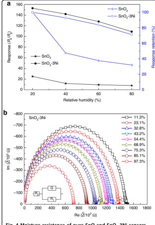
**Fig. 4 Moisture resistance of pure SnO and SnO -3Ni sensors. a** The responses of the sensors based on pure  $SnO_2$  and  $SnO_2$ -3Ni at humidity range from 20% to 80% *RH*; **b** EIS plots of the  $SnO_2$ -3Ni sensor under different humidity conditions
