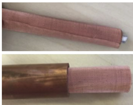
Fig. 10. Wick insertion for the cylindrical containers (Mahdavi et al. [63]). Reprinted from Experimental Thermal and Fluid Science , 93, Mahboobe Mahdavi, Saeed Tiari, Sven De Champheleire, Songgang Qiu, Experimental study of the thermal characteristics of a heat pipe , Pages No.292-304, Copyright (2018), with permission from Elsevier
