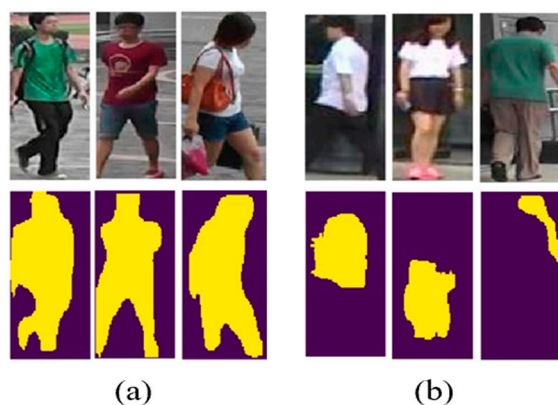
Figure 2. Some results of segmentation masks: (a) Complete; and (b) incomplete. The top row denotes original images, with corresponding binary masks below, where body regions display in yellow pixels.
