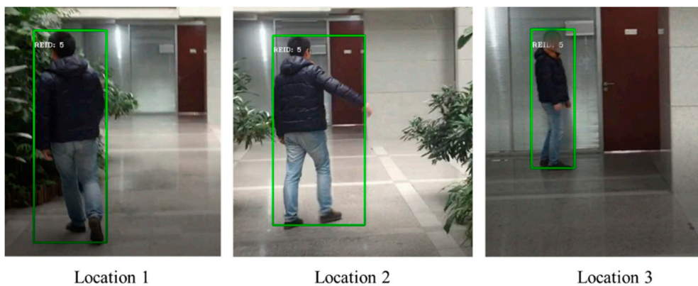
Figure 6. A long period tracking in the view of robotics with DPA model. Our method is applied to help keep following the target person for a long period with interference and occlusion.
