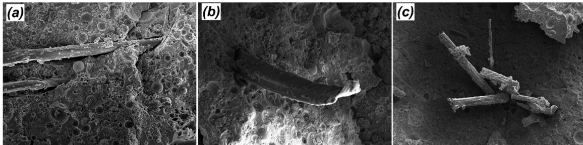
Figure 8. SEM images showing the fracture surfaces of flax fibres reinforced composites; (a) GP/flax fabric (FF), and (b,c) GPNS-1/FF [25].
