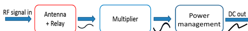
Figure 7. Block diagram of step-up converter and power manager for energy harvesting application.
