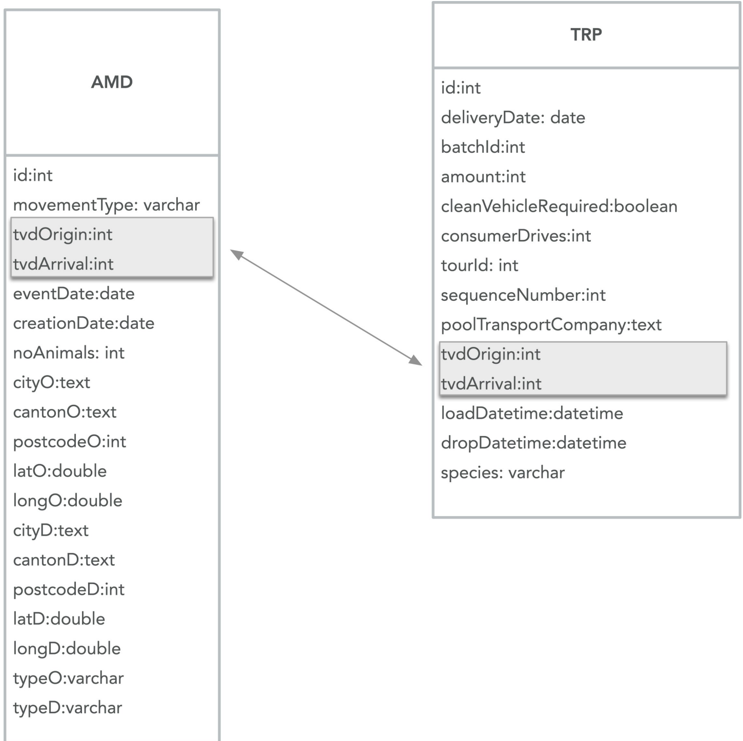
Fig 1. Graphical representation of the raw data we collected from AMD (on the left) and TRP (on the right). The matching of movements is based on the attributes tvdOrigin (integer) and tvdArrival (integer) in both data sets.
