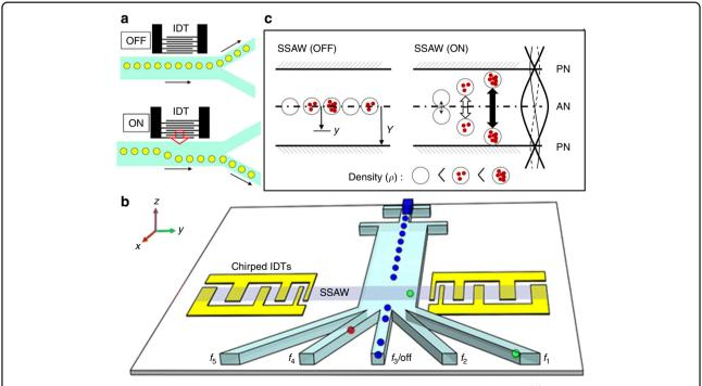
**Fig. 7 Acoustofluidic droplet separation. a** Deflection of droplets by traveling SAW-induced acoustic streaming<sup>141</sup>. Reprinted with permission from the Royal Society of Chemistry. **b** Separation of droplets by changing the frequencies of slanted IDT<sup>142</sup>. Reprinted with permission from the American Society of Chemistry. **c** Separation of cell-encapsulated alginate beads based on density<sup>144</sup>. Reprinted with permission from the AIP Publishing
