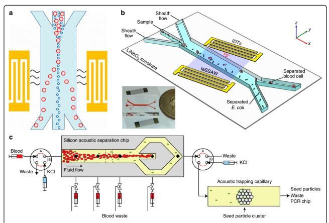
**Fig. 5 Acoustofluidic separation of bacteria. a** Separation of bacteria from blood cells using a standing SAW technique<sup>121</sup>. Reprinted with permission from the American Chemical Society. **b** Blood cells are deflected by tilted-angle SAW field and thus separated from bacteria<sup>122</sup>. Reprinted with permission from the IOP Publishing. **c** Separation and enrichment of bacteria by acoustofluidics<sup>123</sup>. Reprinted with permission from the American Chemical Society
