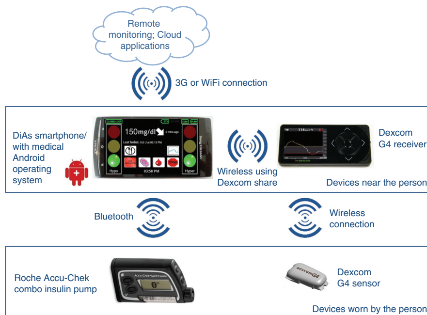
Figure 4. The Diabetes Assistant (DiAs), which became the first portable artificial pancreas (AP). This configuration has been used in several closed-loop control studies: a smartphone using a modified Android operating system, locked to meet medical device requirements, runs the control algorithm, the graphical user interface, and the wireless communications with a continuous glucose monitor (Dexcom G4), an insulin pump (Roche Accu-Chek), and with a remote server (through WiFi or cellular network) that provides real-time monitoring capabilities, analytics, and database support.
