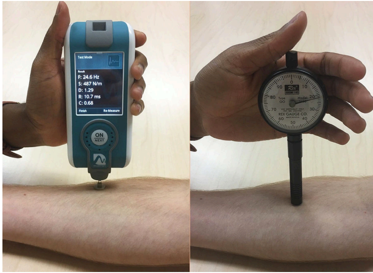
Figure 1: Myoton, a noninvasive handheld device modified to isolate cutaneous tissue, and the Rex gauge OO durometer
