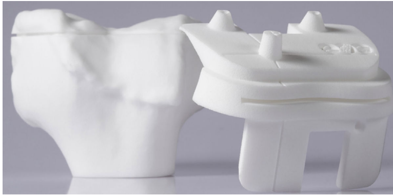
Fig. 5. Nylon 12 EOS PA2200 patient-specific cutting guide fabricated using an LPBF process (EOS P396 machine). ( Courtesy of EOS North America; with permission. )
