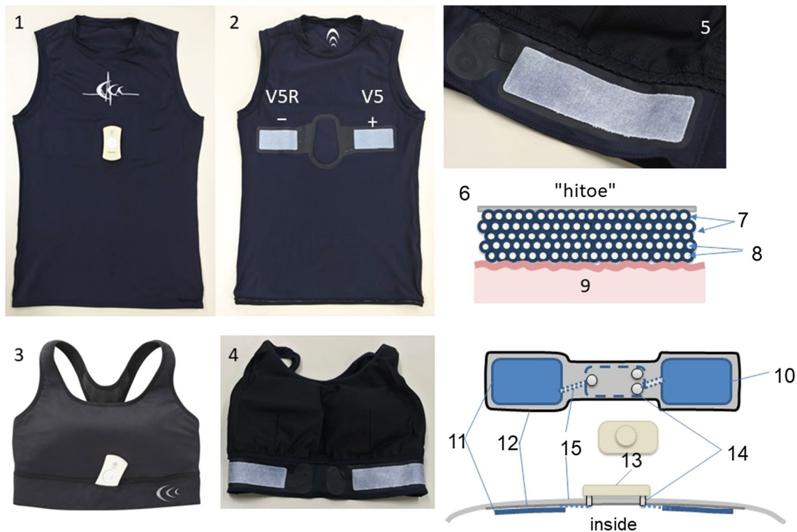
Fig. 1 Wearable ECG of smart garment. The ECG sensor patches (5) were placed inside the undershirt (“1. 2.” outside and inside faces for men or the bra strap “3.4.” for women). (6) Cross-sectional view of the textile electrode (hitoe ® ). The cloth of polyester nanofiber (8) was coated by electroconductive polymer PEDOT-PSS (7, blue circles), which surface was directly placed on the skin (9). Back side of the
