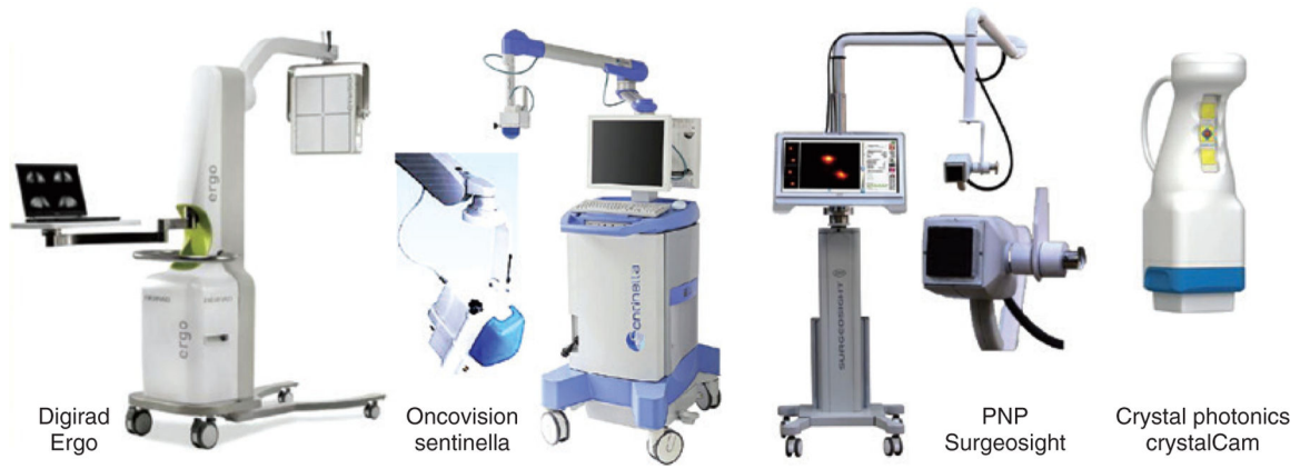
Figure 6. Portable and handheld commercial gamma cameras for intraoperative use. Reproduced with permission from [73–76].
