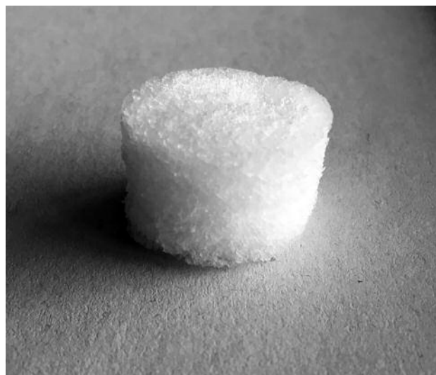
Figure 1. Porous fibroin sponge made after dissolving silk using Ajisawa's reagent and freeze-thawing.
