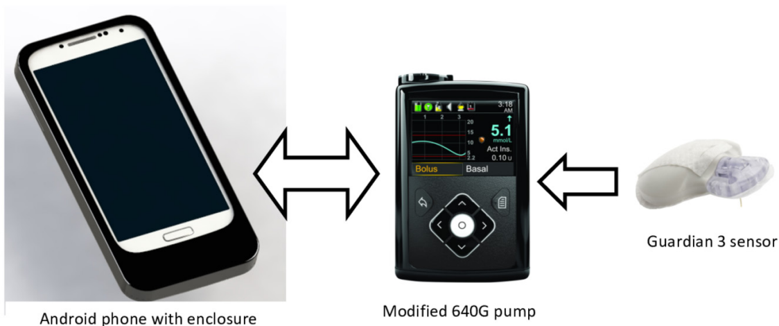
Figure 2 FlorenceM closed-loop system prototype. The system consists of a continuous glucose monitoring transmitter with Guardian 3 sensor (Medtronic), an insulin pump (modified 640G pump, Medtronic) and an Android smartphone running the control algorithm (Cambridge).
