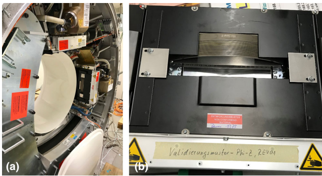
FIG. 10. (a) The prototype of SparseCT with multislit collimator (MSC) installed and (b) a zoomed view of W4S16 MSC. [Color figure can be viewed at wileyonlinelibrary.com ]
